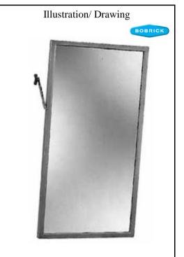
**Frame** — 18-8 S, type 304, heavy-gauge stainless steel, 3/4" x 3/4" (19 x 19mm) angle with satin finish. One-piece, roll-formed construction forms continuous integral stiffener on all sides. Bevel design on front holds frame tightly against mirror. Corners are welded, ground, and polished smooth. Galvanized steel back is fastened to frame with concealed screws. Full-width stainless steel piano-hinge is welded to bottom of frame.
